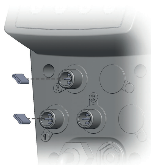
Fig. 9-1: Removing the conductive rubber bands
