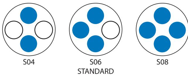
SR-40 and 80 spring return actuators use a minimum of two springs and maximum of seven springs on each side according to the diagram below.
