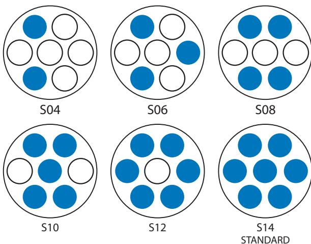
SR-130 to 4000 spring return actuators use a minimum of three springs and maximum of seven springs on each side according to the diagram below.
