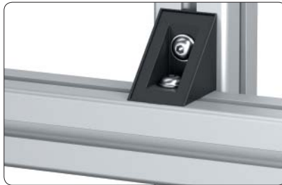
Support across the profile In this application the rotary lock must be removed from one side
