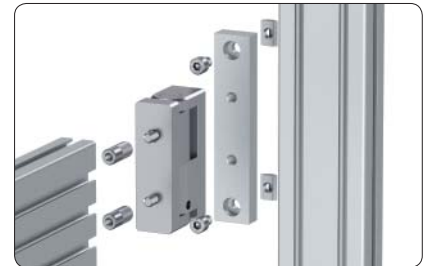
Fastening of profile 30×100 with joint 30×100
